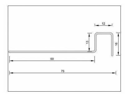
I. Only original JK manufactured "J" bite-bars of thickness 0.8mm to 1.2mm shall be used JK C 43 chassis.
